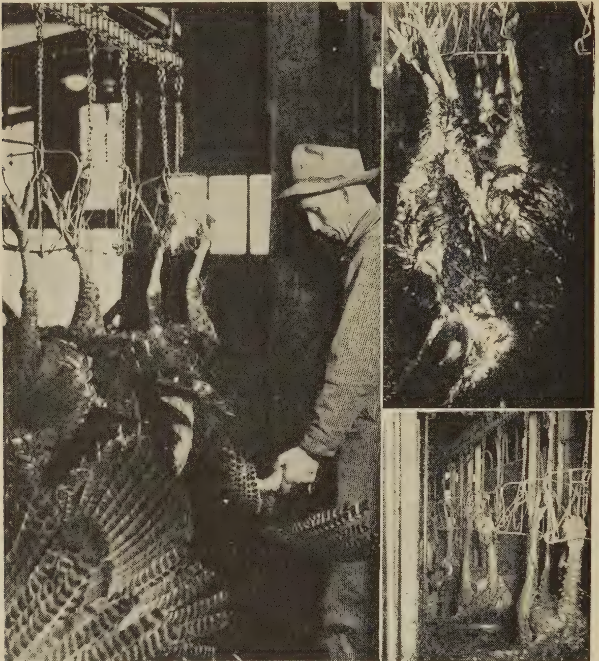
FIG. 157.—(A) Showing various stages in killing and plucking turkeys. Left, the turkeys are suspended from shackles hanging from an endless chain. Note operator ready to kill and bleed a turkey. Top right, the turkeys have been automatically dipped in the slack-scalding tank after having been “roughed.” Bottom right, the birds have been dipped in molten wax. ( Utah Poultry Producers’ Association. )
